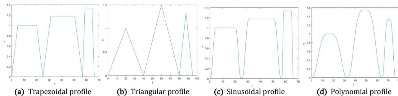
Figure: Sample graphs of velocity for different velocity profiles
