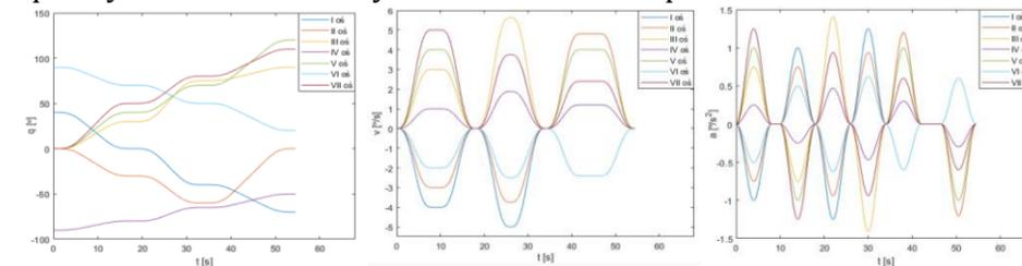
Figure: Positions, velocities and accelerations in axes (sinusoidal profile)
